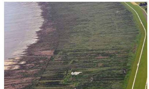
Figure 4.41: Salt marsh of the Jade Bight, Germany. Land reclamation through rows of wooden poles driven into the bay mud leads to a typical salt marsh zonation pattern.
