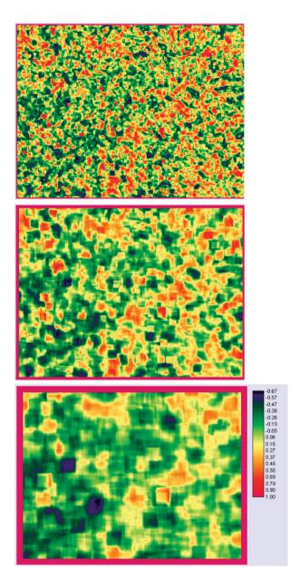
Figure 2. Correlations between environmental characteristics change with spatial resolution. Moving window Pearson correlations between principal components 1 and 2 of a Landsat TM scene for southern Portugal (pixel size  $100\times100$  m). Window size increases from  $500\times500$  m (top), through  $1.1\times1.1$  km (middle) to  $2.1\times2.1$  km (bottom). For the full image (i.e. a single window) the correlation is zero.
